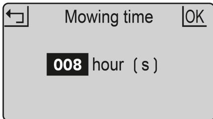
This is the amount of time per day the mower will be active. This includes charging time. For example: if set to 8 hours and the mower is set to operate from 8:00pm it will operate until 4:00am. In this time it may mow for 1 hour charge for 2 hours mow again for 1 hour; charge for 2 hours, mow for one hours and return to charge ready for the next cycle.
